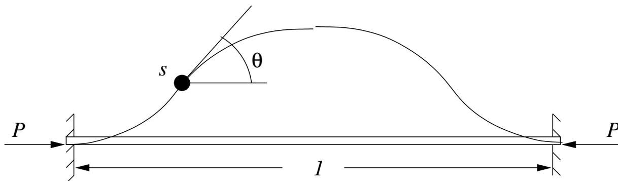
Figure 1: The sketch of the deformed rod geometry
