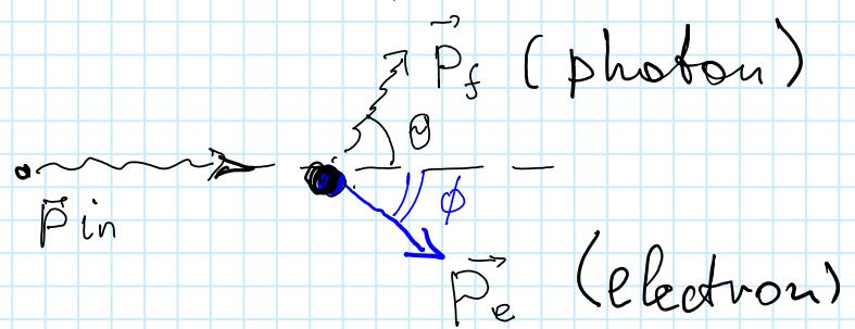
Calculate the energy of a scattered photon as a function of the scattering angle  $\theta$ .
