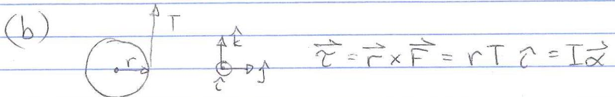
Torque and angular acceleration Vectors II
