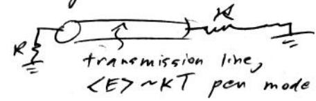
$$\frac{V_{\text{noise}} (\text{rms})}{\sqrt{\text{bandwidth (Hz)}}} = \sqrt{4kTR}$$
