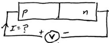
$V$  will appear across depletion region, reducing potential to  $V_0 - V$  (or increasing, if  $V$  is (-)).
