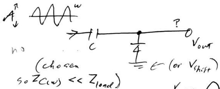
When diode conducts, C charges. So its voltage builds up until conduction stops:
