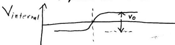
Holes and electrons recombine at boundary until the potential inhibits further net motion.
