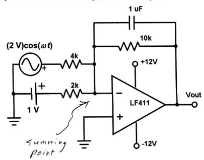
For the IVDC input, the capacitor doesn't contribute, so  $V_{out}/V_{in} = -\frac{10K}{2K}$ , and  $V_{out}, dc = -5V$ .
