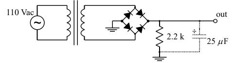
Measure the ac output voltage of the transformer using a DMM set to ac Volts. DO NOT try to measure the voltages across the transformer by connecting the scope ground to one of the transformer coils – they are not at ground. However, the output is perfectly safe to measure. Sketch (or record) and explain the waveform that you see. Why is this the first step in building an ac powered dc power supply? What is not yet satisfactory about the output?
