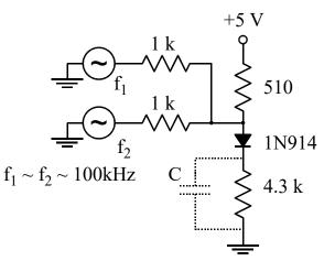
both to limit the bias current and to sample the current through the diode.
