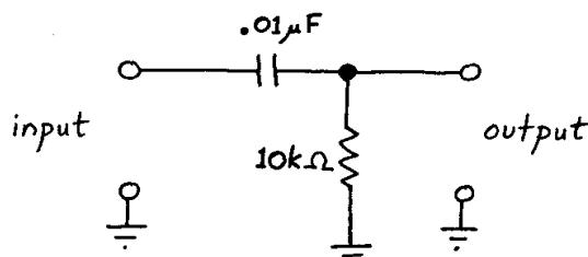
The figure is simple four-terminal RC high-pass filter.
