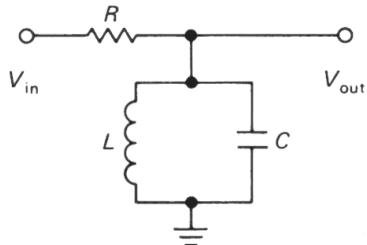
The figure is a simple four-terminal RCL tank circuit. The inductor has a series resistance  $R_L$  and the capacitor has a parallel resistance  $R_C$ .
