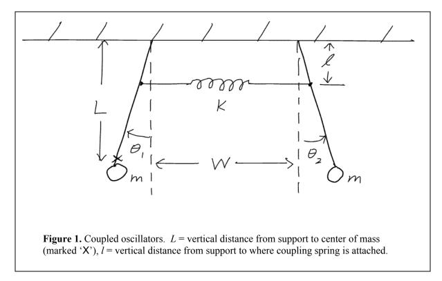
Consider the two identical pendulum bobs displayed in Fig. 1. Without the coupling spring, the small-amplitude motion of either pendulum is described by
