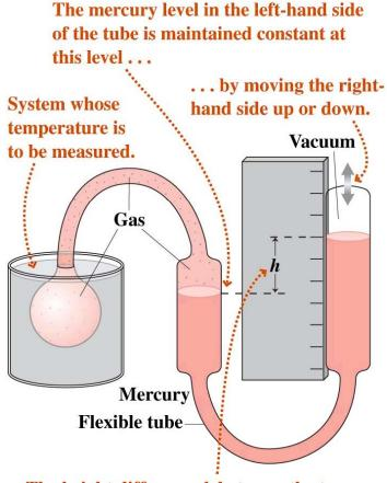
The height difference *h* between the two mercury levels is a measure of the gas pressure and therefore of the temperature.
