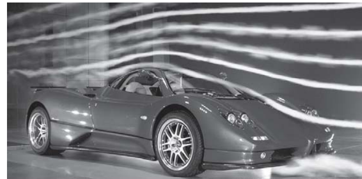
Streamlines in an automobile wind-tunnel test
