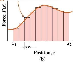
The exact value for the work is the area under the force-versus-position curve.
