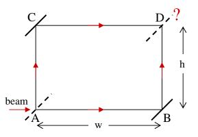
are at right angles and lie in a plane. For the purpose of this problem, the Bragg mirrors may be treated as ideal planar interfaces of negligible thickness.
