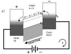
electrodes, but provides an impenetrable barrier to electrons of lower energies.
