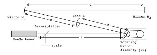
FIG. 1: Diagram of the experimental apparatus used for the measurement of the velocity of light.
