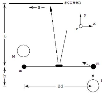
FIG. 2: The rotation of the rigid dumbbell in the  $xy$  plane will cause the position of the reflected light beam to move across the viewing screen.
