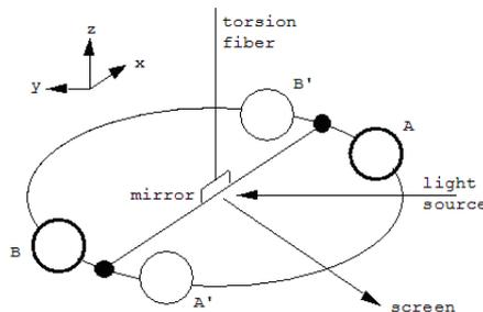
FIG. 1: The two large spheres of mass  $M$  are initially at the positions A and B. The two small spheres have a mass  $m$  and comprise the torsion balance.
