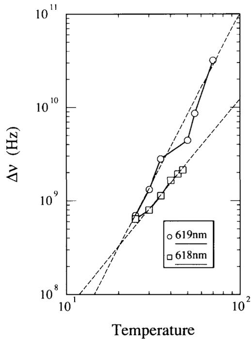
Fig. 3. Homogeneous line widths of  $\text{Pr}^{3+}$  in a  $10^{-6}$   $\text{Pr}^{3+}$  doped silica glass fiber at two different excitation wavelengths.
