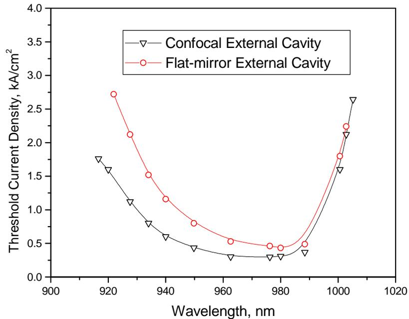
**Figure 2.** Comparison of the threshold current density characteristics of the flat-mirror cavity and the confocal cavity. Confocal cavity has lower loss and wider tuning ability under the same pump current.
