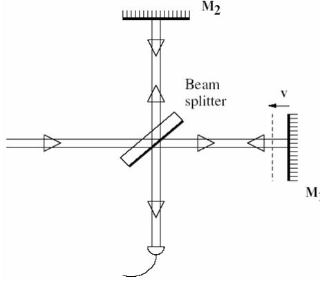
**Figure 2.** A Michelson interferometer (MI) in “filter mode” implying that it is illuminated by a collimated beam and the MI is aligned to generate the output beam as perfectly coincident on the beam splitter and emerging collinearly.
