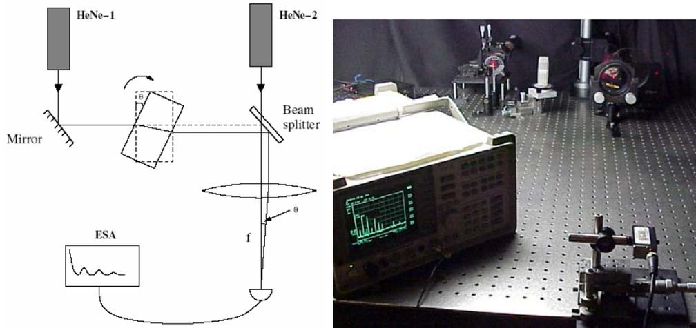
**Figure 4.** An experimental set up and the actual photograph to measure the angular sensitivity of heterodyne beat signal when two beams carrying different frequencies are combined on a fast detector.
