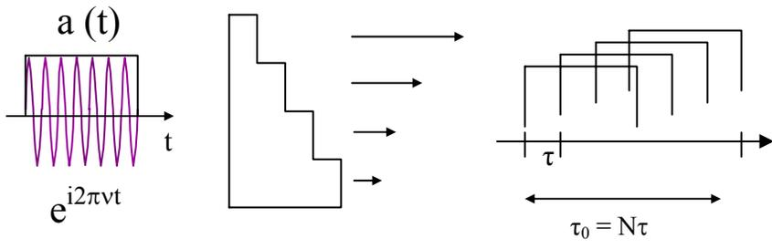
Figure 3. This schematic diagram depicts the partial superposition of a train of finite pulses with a periodic step delay of  $\tau$  produced by an echelette grating. The carrier frequency,  $\nu$ , of the E-vector and the time-finite duration of the input amplitude,  $a(t)$ , is depicted on the left. Notice that all spectrometers have a characteristic time constant for its fringe evolution, or pulse stretching, given by  $\tau_0 = N\tau$  [13].
