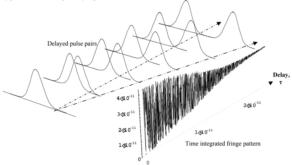
Figure 5. Variation of long-time integrated, fringe visibility in a simple Michelson interferometer as the delay between the mirrors is varied. The pulse,  $a(t) \exp [i2\pi\nu t]$ , is considered perfectly reproducible and the time integrated fringe energy is recorded separately for each delay position,  $\tau$ . The resultant visibility of the fringes, degraded by  $\gamma(\tau)$ , is due to superposition of unequal amplitudes on the detector.
