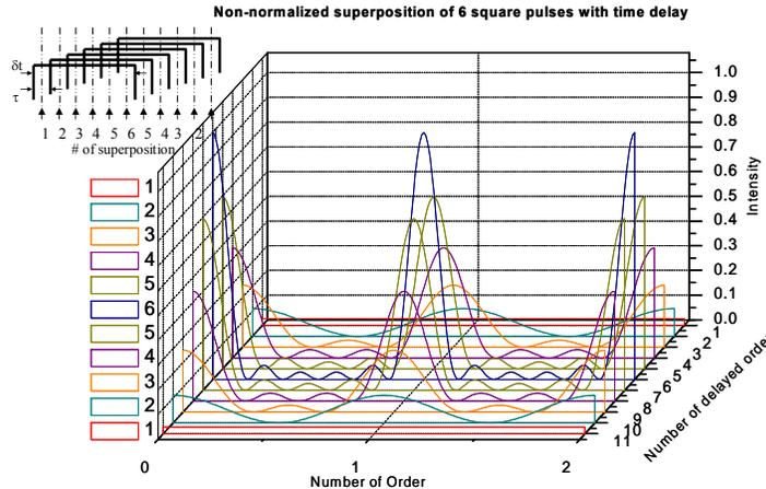
Figure 4. Time evolving fringe width due to a single rectangular pulse transmitted through a Fabry-Perot interferometer. The number of superposed pulses increases with time, producing narrower fringes. The process then reverses with fringe broadening again. When a photographic plate integrates all these time varying fringes, we get a broader interference fringe compared to a CW illumination with the same carrier frequency [13].
